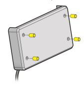
Place the LGT-B10 over the brake pedal plate with the wire at the bottom.
