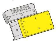
Push <u>Spacers</u> in the (4) holes of the new LGT-B10 brake pad.
